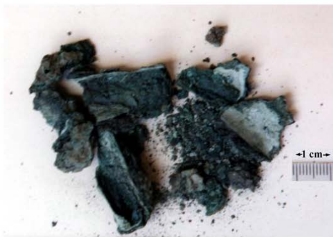
Figure 2. Bronze scabbard (L84-85) decayed due to attack by copper chlorides.
