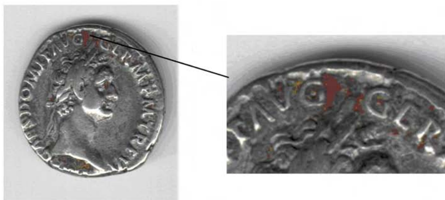
Figure 14. Denier of Domitian (S894) with the red outgrowth corresponding to cuprite.
