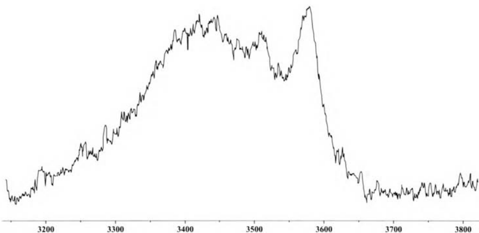
Figure 18. Raman spectrum at high wavenumbers: standard sample of ZnO (CAZN09).
